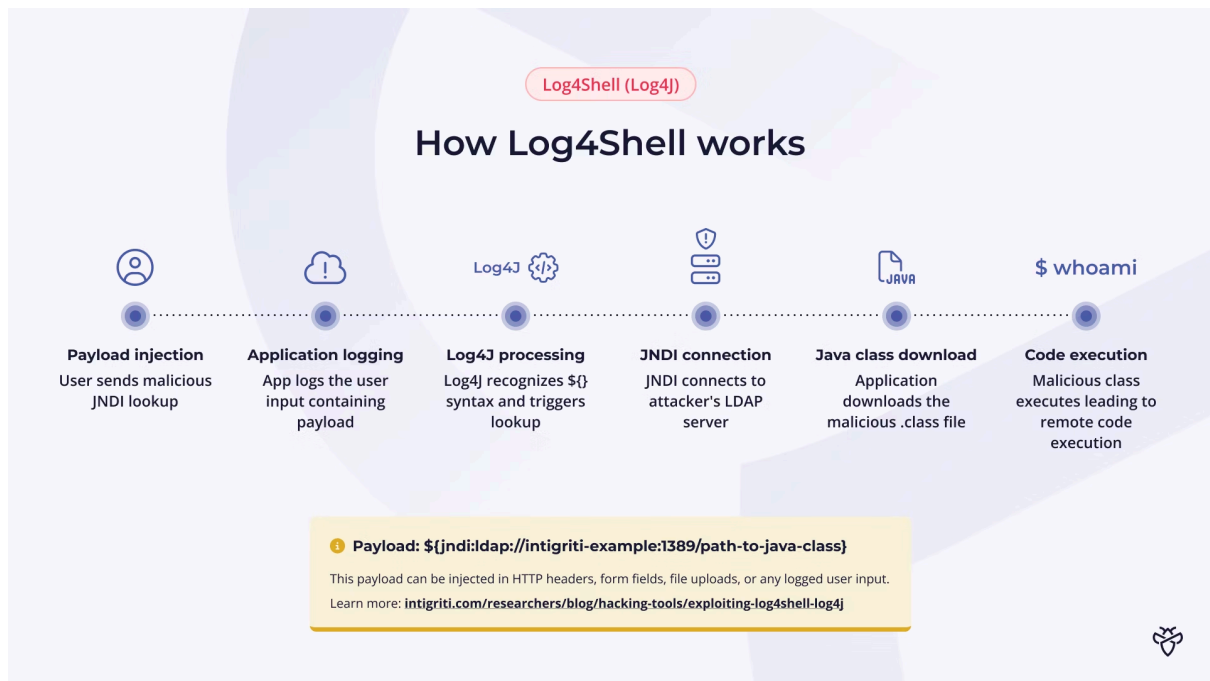
How the Log4Shell (Log4J) exploit works
